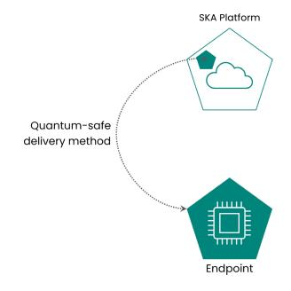
Registration relies on the quantum-safe delivery of a root key, called the bootstrap key, to every device. There are several possible methods for safe bootstrap key delivery depending on the device and the environment. Delivery methods include both manual delivery of keys and overthe-air. Once the bootstrap key is installed a device registers with SKA Platform via a simple API call.
